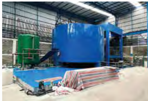
KAI ALLUMINIUM LTD ETP (capacity 600 m 3 /day)
